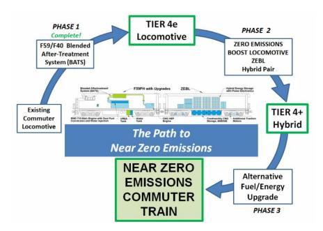
This chart shows how Rail Propulsion Systems' research and development project will upgrade any locomotive to a zero-emission, batteryoperated hybrid locomotive. Image from <u>www.railpropulsion.com/path</u>
